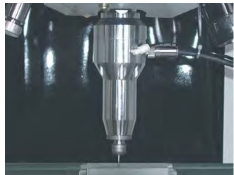
HES510 Spindle - Max. 50,000rpm HES810 Spindle - Max. 80,000rpm
